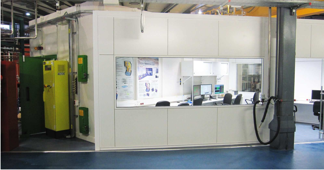
Figure 1. BL22-CLAESS: BL22's control cabin. The green door at the left is entrance to the experimental hutch. The photograph was taken at the entrance to the Chemistry Lab that will be used for sample preparation/mounting.
